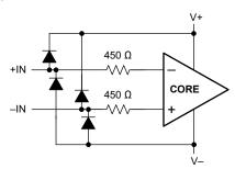
Figure 7-1. Equivalent Input Circuit
