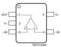
Figure 5-1. OPA387: DBV (5-Pin SOT-23) Package, Top View
