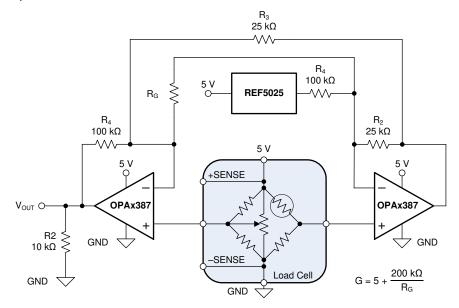
Figure 8-3. Load Cell Measurement Schematic
