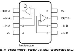
Figure 5-2. OPA2387: DGK (8-Pin VSSOP) Package, Top View
