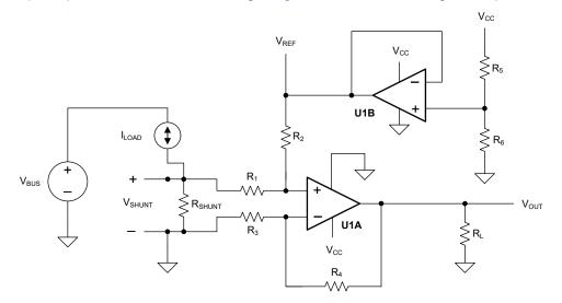
Figure 8-1. Bidirectional Current-Sensing Schematic
